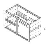
The 2 HP wide front panel covers an open slot. The U-profile front panel can be combined with a textile EMC gasket. It be fixed with screws and washers. Due to the 2 HP width no sleeves can be used.
