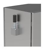
The side mounting kit allows for a vortex cooler to be installed in the field and in many different positions outside of the enclosure, which means it can be used in many different applications. Without this kit, the vortex cooler can still be installed in the field, but only on the enclosure's roof.
