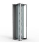
These vertical profiles and rear cover, MSSB, form the basis for plug-in sections. This accessory is available off the shelf and is tested according to IEC 61439. The cover prevents staff from coming into contact with the busbar and the plug in system allows for the compartment to be extracted without turning off the power.
