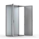
The stainless steel double door combinable floor standing enclosure range, MCDS, is ideal for installation in confined spaces where a single door, when opened, would take up too much space in front of the enclosure. The doors' loading capacity also increases as it is divided over two doors. With a IP 55 protection degree, components inside the enclosure are well protected and makes it well suited for almost any environment, grade dependent.
