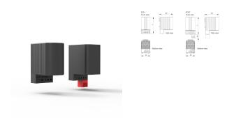
This double insulated compact heater, ECH(T) is available with or without a thermostat. Water condensation is eliminated, also when the ambient temperature drops sharply. Choosing a version with an already integrated thermostat will save space inside the enclosure and reduce installation time compared with a thermostat mounted separately.
