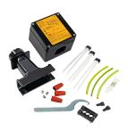
nVent RAYCHEM T-100 is a cold-applied high profile splice or tee connection kit for trace heating cables in both non-hazardous and hazardous locations. Mounted on the pipe, through the thermal insulation and cladding. Includes coldapplied heating cable core sealer.
