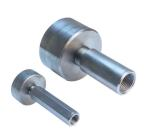
The nVent LENTON D14A Mechanical Anchor with Extension provides a method of splicing and anchoring reinforcing bar in segmental concrete construction applications that have limited space or are severely congested. The large head significantly reduces required embedment lengths. The anchors are a combination of standard nVent LENTON Terminator D14 Mechanical Anchors and ELFM Female-to-Male Extensions.
