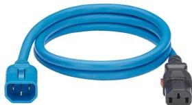
Secure dual W-Lock power cords provide enhanced cord retention between both the PDU and IT equipment. Both connections require deliberate action in order to release the locking buttons to prevent accidental detachment of power connections. Cords function with any corresponding standard IEC receptacle, but locking feature requires compatible W-lock or V-lock outlets
