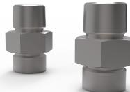
This plumbing adapter is a male-male fitting with 1" BSPP flat seal thread on one end and 1" NPT on the other. It adapts the BSP style 1" hoses for installation in US style NPT chilled water facilities.
