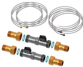
The stainless steel pipe inserts with ID 1" each come with a pair of ratiometric liquid coolant sensors. The sensors connect directly to the RackChiller Rear Door Controller. This enables monitoring of the coolant thermal properties and cooling performance, as well as additional temperature control features.
