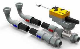
The flexible hoses package for RDHX Pro connects the cooling device to facility water system. The high quality EPDM hoses perform with excellent chemical stability with typical water and glycol based cooling media. The steel reinforcement provides extended pressure capability with rated nominal pressure 5 bar and minimum burst pressure 20 bar, while the external layer protects the hoses from mechanical stress and damages.
