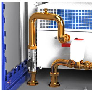
The stainless steel pipe inserts with ID 1" each come with a pair of ratiometric liquid coolant sensors. The sensors connect directly to the RackChiller Rear Door Controller. This enables monitoring of the coolant thermal properties and cooling performance, as well as additional temperature control features.
