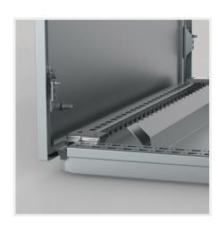
**Description:** Replaces two parts of the standard three or four piece bottom plates. Due to the hammer head cones, EMI cables can be directly earthed to the bottom plate keeping the "Faraday cage".
