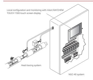
nVent RAYCHEM distribution panels are specially designed to power, control and monitoring electrical heat tracing circuits. The system offers a complete standard set of configurations, serving most heat-tracing applications. The panels vary from power distribution panels up to systems with full control and monitoring capability. The panels are available with a combined incomer or with a separate incomer section.
