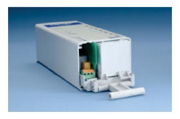
Wire to alarm terminals through gland and replace mounting plate. Permissible wire size is #24-16 AWG (0.2 - 1.5mm2) Remote Status Indicator Dry Contacts are rated at a peak load voltage of 600VAC, a max continuous load current of 0.05A, and max 0.15A peak load current.
