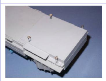
Step 2: Turn over, and remove the four screws holding the fuse cover in place. These screws are tight - use correct screwdriver size to avoid damaging screw head.
