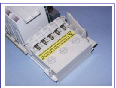
Step 3: Use a large flat blade screwdriver to turn the appropriate fuse ejector a quarter turn (90 degrees).
