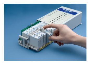
Step 2: Slide out the internal "tray" using the handle located behind the end mounting plate. Replace any failed surge protection module with the correct module type. (Note: must replace with identical part number and voltage rating, contact your local ERICO representative for replacement module ordering advice.
