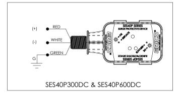
For 3-Phase, 4-Wire 480V WYE (no neutral) systems or 3-Phase 240V and 480V DELTA systems, cut neutral wire and cap.
