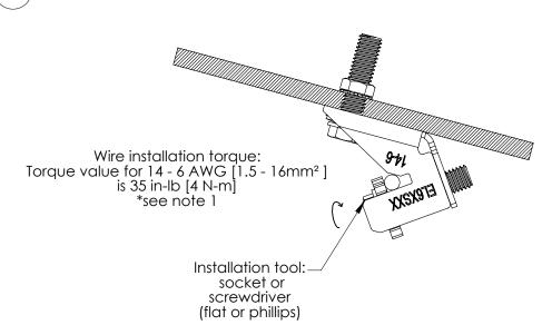
Note: Torque value for 14 AWG stranded [1.5 - 2.5mm<sup>2</sup>] is 15 in-lb[1.7 N-m]
