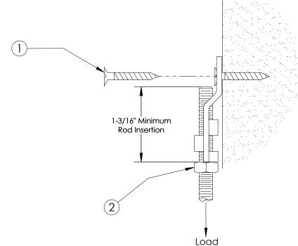
A structural attachment used to join hanger rod to a structure.
