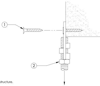
A structural attachment used to join hanger rod to a structure.
