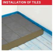
Tiles are placed directly on top of the Reflecta plates with tile adhesive, according to the instructions.
