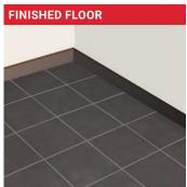
Seal tiles with silicone. Allow the floor to cure completely before turning the underfloor heating system on.
