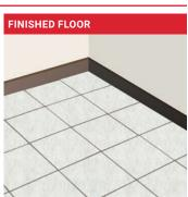
Seal between the natural stone and walls with a silicon sealant. Allow the floor to cure completely before turning the underfloor heating system on.
