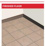
Seal between tiles and walls with a silicon sealant. Allow the floor to cure completely before turning the underfloor heating system on.
