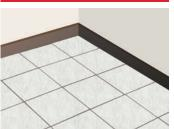
Seal between the natural stone and walls with a silicon sealant. Allow the floor to cure completely before turning the underfloor heating system on.
