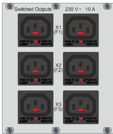
IEC 60320-C13 locking outlets
