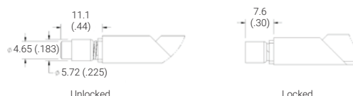
Detail "V" Provides visual lock indication.
