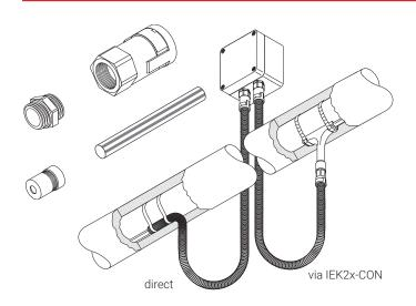
This connection kit is designed for terminating the full range of nVent RAYCHEM XPI polymer insulated series heating cables and cold leads in to a junction box, as well as providing a reliable and sealed connection to a conduit system.
