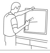
3. Recoat the filters with RP Super Filter Coat adhesive. When spraying filter do so from both sides for maximum concentration of adhesive.
