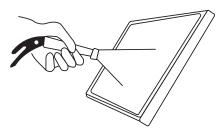
1. Flush the filter with warm water from the exhaust side to the intake side. Do not use caustics.
