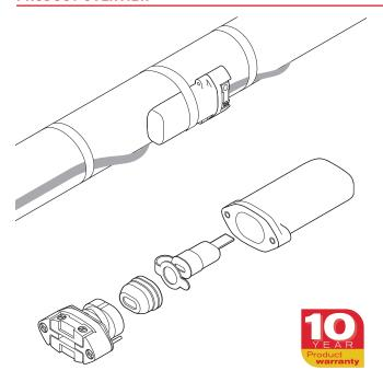
The nVent RAYCHEM E-150 is a cold-applied low-profile end seal. It is designed for use with the following nVent RAYCHEM brand heating cables: BTV, QTVR and XTVR. Use the E-150 in applications with temperatures ranging from -60°F to 420°F (-50°C to 215°C). It is approved by FM, CSA, and Dekra for use in hazardous locations.
