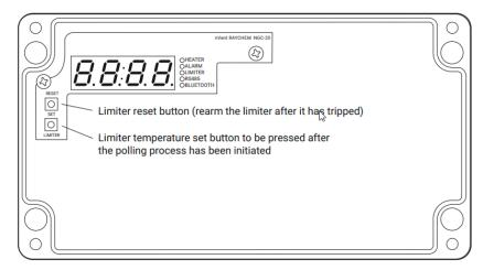
Figure 13-5: Location of "Set" and "Reset" Buttons on NGC-20 Controller
