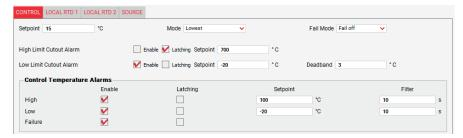
Figure 10-3: Temperature Screen, Control Settings
