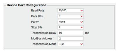
Figure 14-3: Setup Screen, Device Port Configuration
