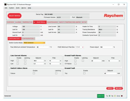
Figure 7-7: Save pending changes with the Apply Button
