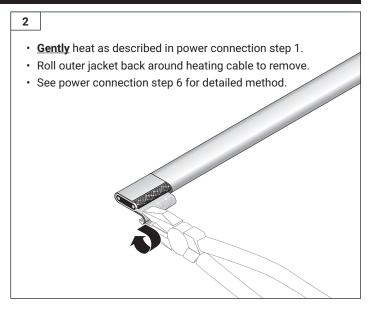
cables' outer jacket. · Ensure no remaining braid wire fragments. · Be careful to not damage inner jacket.
