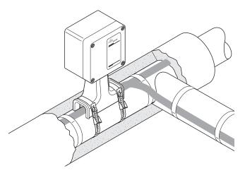
The Raychem T-100 serves as an above-insulation splice or tee for up to three Raychem brand BTV, QTVR, XTVR, HTV or VPL heating cables. It is approved for use in hazardous locations.
