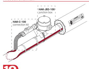
The nVent RAYCHEM HAK-C-100 connection system is FM approved for use with nVent RAYCHEM HBTV, HQTV and FHP heating cables in Class I, Division 1 hazardous locations. It is also CSA certified for use with nVent RAYCHEM BTV-CT, QTVR-CT, XTV-CT, VPL-CT, and LBTV2-CT heating cables and c FM us approved for use with nVent RAYCHEM HTV heating cables in Class I, Division 1 locations.
