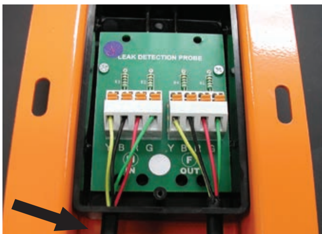
Figure 3. Multiple probe wiring configuration and suggested tie wrap location
