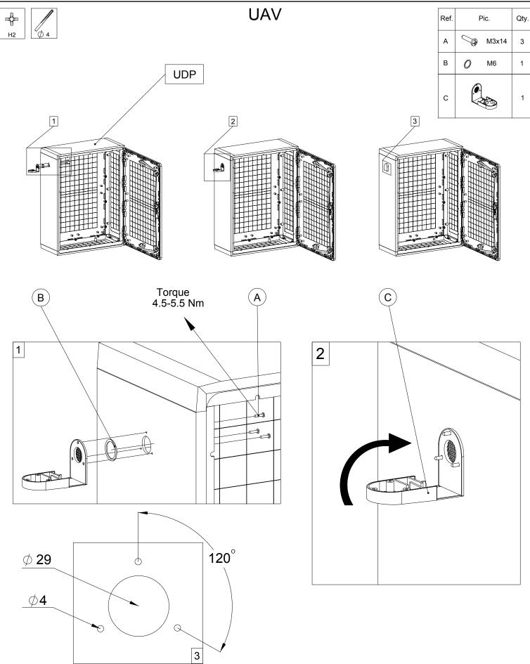
It is highly recommended to install two air vents per enclosure for sufficient air circulation.
