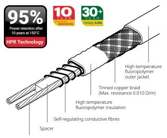
2.3 mm<sup>2</sup> nickel plated copper conductors
