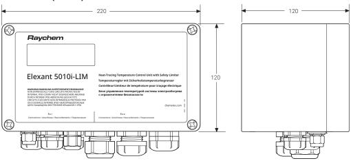
Sample shown is Elexant 5010i-LIM. Gland included in scope of delivery - 1 x M25 x 1,5
