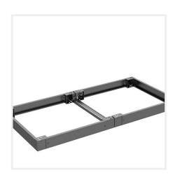
**Description:** Acts as a stabiliser when cabling is routed between bayed enclosures. With the PCP, plinths can be combined and fixed to the floor before the enclosures are mounted on them. The PCP can be used when cables have to go under the enclosure. For 200 mm high plinths, the PCP can be mounted in three different heights, top, middle or bottom. The hole pattern for cage nuts and M5x10 screws, allows accessories to be mounted.
