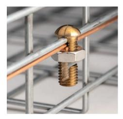
nVent ERICO Lay-in Split Bolt is a high-strength corrosion resistant alloy bolt engineered with a round head design to prevent damage to wires plus includes a captive nut and saddle, allowing for no loose hardware. It is ideal for high-volume installations, providing an easy, time-saving, one-handed installation.
