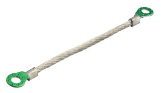
nVent ERICO PermaGround Surface Bonding Jumper is a conductor used to ensure electrical continuity and a lowimpedance path for fault currents between metal parts that need to be electrically connected.
