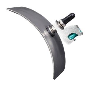
nVent ERICO PermaGround Pool Bonding Kit is made up of stainless steel and designed to create an equipotential bond around a swimming pool, ensuring all conductive parts of the pool area, including the water, are at the same electrical potential, minimizing the risk of electrical shock.
