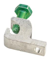
nVent ERICO PermaGround Lay-In Ground Lug is an electrical connector engineered for easy and efficient grounding. It's open-faced design allows the grounding conductor to be "laid in" without the need to thread it through a closed connector, simplifying installation.
