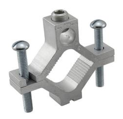
nVent ERICO PermaGround Water and Gas Pipe Ground Clamp is engineered of high-strength 6061-T6 aluminum alloy and are used for connecting copper or aluminum conductors to copper water pipe, galvanized pipe or steel conduit. The conductor and pipe range taking capabilities make this connector ideal for installations requiring long ground wire runs.
