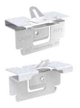
The nVent CADDY T-Grid Clip for Recessed Light Mounting Bracket is a spring clip that allows contractors to connect the recessed light adapter to a T-Grid application. Quickly snap the Clip onto the Telescoping Recessed Light Mounting Bracket without the need to screw onto a T-grid. Contractors can rest assured that lights are easily positioned within the T-grid application, ensuring less time spent on the ladder during installation.
