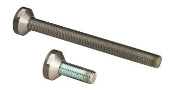
The nVent LENTON Interlok No-Thread Bar Positioner provides a hard stop to prevent the over-insertion of rebar during pre-cast installations. Designed for use with the nVent LENTON Interlok No-Thread Grout-Fill Coupler, this robust system ensures secure and accurate placement with every use. Both easy-to-install and remove, the Interlok No-Thread Bar Positioner is reusable with minimal wear and tear, ultimately saving valuable time and money on the job site.
