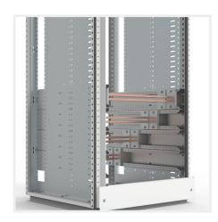
**Description:** Support to be mounted horizontally in the enclosure. Is mounted to the internal side panels, MSPS, and the enclosure frame. Makes it possible to mount the MSHS busbar support in depth in a horizontal position. Ideal when there are many incoming/outgoing cables and need a horizontal connection.
