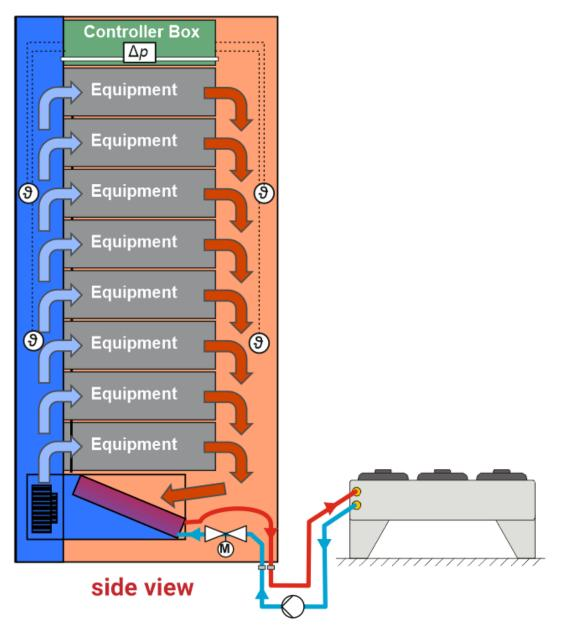
The water inlet temperature and the cooling water flow and the air flow determine the cooling capacity of the cooling module.
