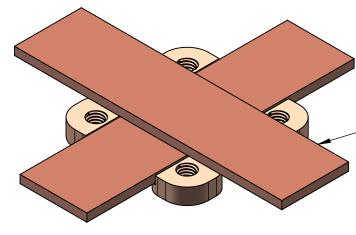
3: Insert the second copper tape in right angle to make a X connection (B1)
