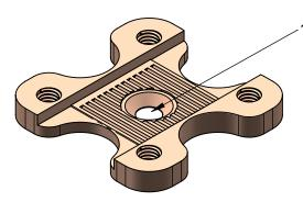
1: Screw this part on support with a countersunk screw M6 (the screw is not provided)
