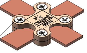
4: Place the second part of the piece and Screw this part at 5 Nm max with the 4 x M6 countersunk head pozidriv screw included
