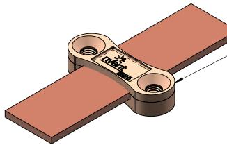
4: Screw this part to close the fixing with the 2 M6 pozidriv countersunk head screw included at 5 Nm
