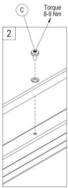
$<sup>^{\</sup>star}$  - Used on enclosures 800 mm deep. \*\* - Torque value for first tightening. For following tightening, torque value recomended is 4-5 Nm.
