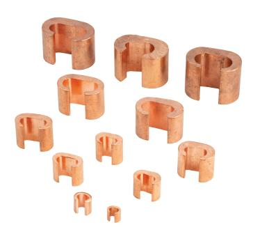
The nVent ERICO PermaGround Compression Connector, C-Crimps are high-strength, conductive copper connectors designed to create permanent, low-resistance grounding connections. These C-Crimps utilize a compression tool to join two grounding conductors securely, and their range-taking design accommodates various conductor sizes. Clear markings and all-weather durability make them ideal for diverse applications, including direct burial.
