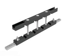
**Descripción:** Busbar support up to 1600A to be mounted horizontally or vertically. Mounts directly to the enclosure frame or with help of CLPF profiles. Available in single and double bar per phase for bar thickness 5 mm and only single bar per phase for bar thickness 10 mm, and width from 25 to 80 mm.
