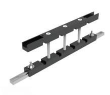
**Descriere:** Busbar support up to 1600A to be mounted horizontally or vertically. Mounts directly to the enclosure frame or with help of CLPF profiles. Available in single and double bar per phase for bar thickness 5 mm and only single bar per phase for bar thickness 10 mm, and width from 25 to 80 mm.
