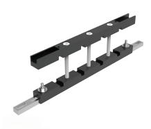
**Descrição:** Busbar support up to 1600A to be mounted horizontally or vertically. Mounts directly to the enclosure frame or with help of CLPF profiles. Available in single and double bar per phase for bar thickness 5 mm and only single bar per phase for bar thickness 10 mm, and width from 25 to 80 mm.
