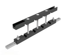
**Opis:** Busbar support up to 1600A to be mounted horizontally or vertically. Mounts directly to the enclosure frame or with help of CLPF profiles. Available in single and double bar per phase for bar thickness 5 mm and only single bar per phase for bar thickness 10 mm, and width from 25 to 80 mm.
